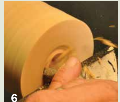
6 Refine the mouth of the vase using a sharp bowl gouge with light cuts.
