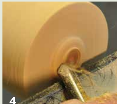
4 Remove the tailstock support and clean up the remaining area, taking light cuts. Establish a center point using a skew chisel.
