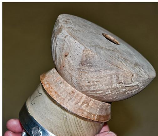
After the exterior is finished, the hollowing process begins. After the initial hollowing, Steve used a captive bar hollowing rig to complete the hollowing process.
