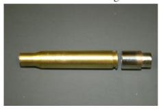
bushing for some other project that is the correct size. I have also made bushing by take an aluminum or cold rolled steel bar and drilled a hole to fit the mandrel shaft. I then turned the metal down to final size using high speed wood turning tools. High speed steel is what a machinist would use to turn aluminum or soft cold roll steel. The
