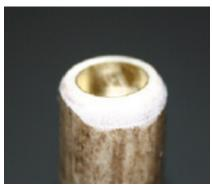
piece from the mandrel and place it between the wooden drive taper and the live center. Sand the piece and fill any porous material. Finish as before.
