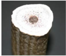
of the piece as possible. This hole will be the guide for all the other drilling to come. I take the piece to the lathe and mount it between the wooden taper and live center. Using a roughing gouge, I round the piece enough to easily fit in the spigot jaws of a chuck. Leave some rounding for the final turn-
