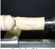
ing as the chuck will leave indentions in the antler that will need to be removed later. Now place one end of the piece in the spigot jaws of a chuck. Use the live center in
