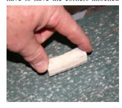
off. I very carefully hold the piece on the end with my thumb and first finder and place on a belt sander. Belt sanders can remove skin very quickly. I will form as many flat surfaces as I can on up to four sides. This should help the piece
