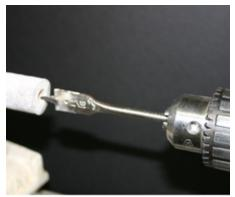
not to hit the four jaw chuck at the far end. The holes for the screw on caps are made with a 13/16 in. forstner bit (\$10). Before you drill the hole, clean up the end and make sure it is square to the lathe. Now drill a hole about inch deep. Re-
