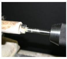
move the piece and mark it for final length. Reverse the piece in the four jaw chuck with the drilled end toward the jaw. Center with the live center and tighten the chuck. Turn the end to final length and square up the end. Drill a inch deep hole with the 13/16 forstner bit.
