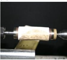
off the ends. Be sure to remove and marks left by the four jaw chuck.
