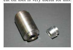
I slowly rock the tool left and right and take off metal until I have a bushing. The tools that I have the best results in turning antler are roughing gouges and spindle gouges. I do not get good results using a skew or scraper. Slowly turn the antler down to final size to match the bushing size on the ends and a
