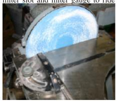
in the slot. The miter gauge must be at a 90 angle to the sanding disk. This is easy to check with a plastic 'square'. I make blocks of wood that can ride against the mi-
