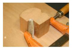
slowly and remove the bit often to clear the antler that tends to clog the drill bit. After completing the drilling, remove the piece and carefully check to see that the drill bit did not blow out the side or bottom. You are now ready to glue the tube.
