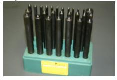
at Harbor Freight for about \$15. Find a punch that just fits snuggly inside the pen tube. Find a drill bit slightly smaller than the punch or the same size as the punch. Turn the 4x4 block up on end on a drill
