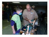
sisting that each student wear safety glasses and a dust mask while working at the lathe. The students then
