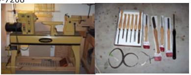
**Powermatic 4224** Power is 3 hp single phase 220v. Lathe capacity is 24" dia. x 42" long.
