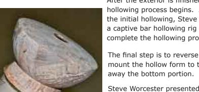
After the exterior is finished, the hollowing process begins. After the initial hollowing, Steve used a captive bar hollowing rig to complete the hollowing process.
