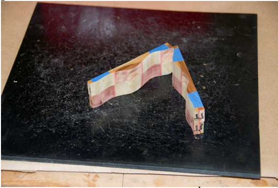
Pic 11: Inside of blanks after 2 nd cut
