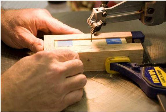
Pic 1: Cutting a curve using L-shaped push blocks
