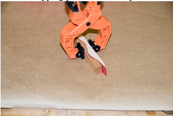
Pic 5: Temporary clamp keep parts aligned
